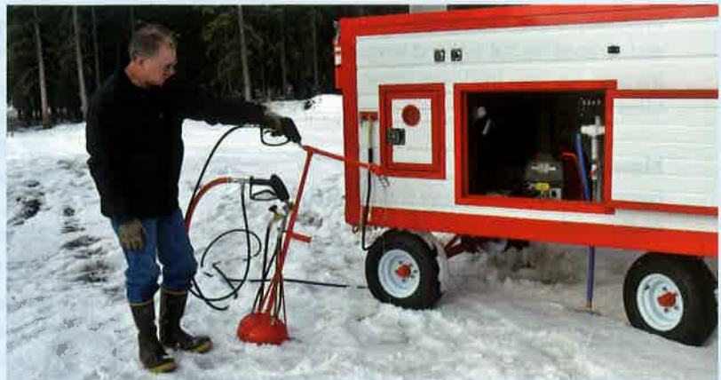
The support trailer is designed for towing by snowmobiles and all-terrain vehicles.
